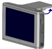
GPS Antenna Up (Parallel to the Ground)
